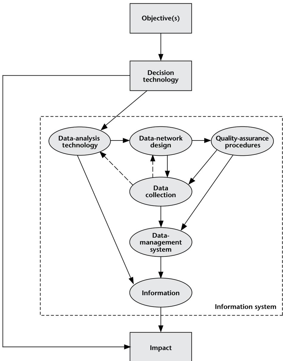
Figure I.2.2. Components of a hydrological information system
