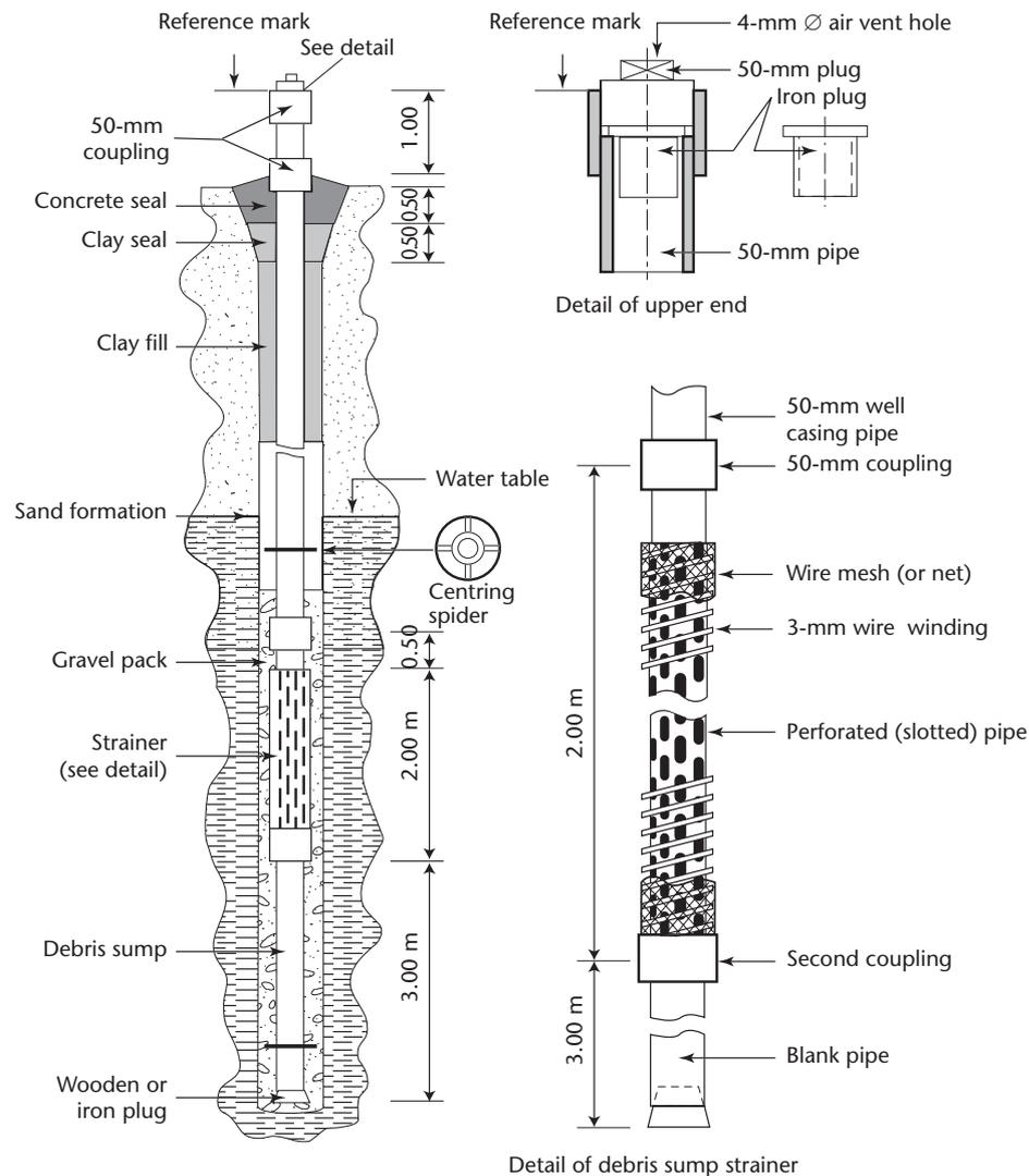
**Figure I.6.3. Observation well in a sand formation**
