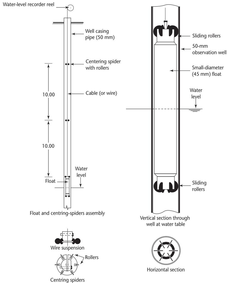
Figure I.6.5. Small-diameter float with sliding rollers in an observation well
